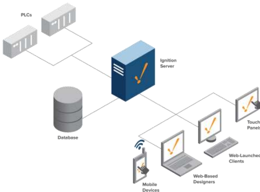
Figure 1. SCADA system architecture and communication structure.
